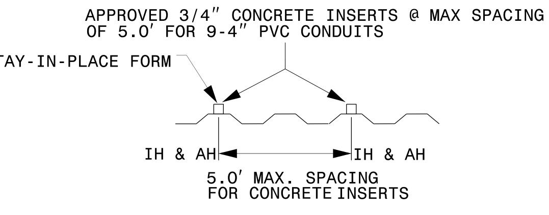
EXACT SPACING MAY VARY IN ORDER TO AVOID LOCATING INSERTS ON SLOPING OR LOW SURFACE OF STAY IN PLACE FORM.
