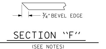
EMBEDDED PLATE "B-1" DETAILS FOR AASHTO TYPE III GIRDER (2 REQ'D PER GIRDER)
