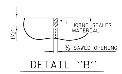
A  $1\frac{1}{2}$  DEEP,  $\frac{3}{8}$  WIDE CONTRACTION JOINT AT BENT CONTROL LINE SHALL BE SAWN WITHIN 24 HOURS OF POURING THE DECK. THE JOINT SHALL BE FILLED WITH JOINT SEALER MATERIAL. THE JOINT SEALER MATERIAL SHALL CONFORM TO THE REQUIREMENTS OF SECTION 1028-3 OF THE STANDARD SPECIFICATIONS.
