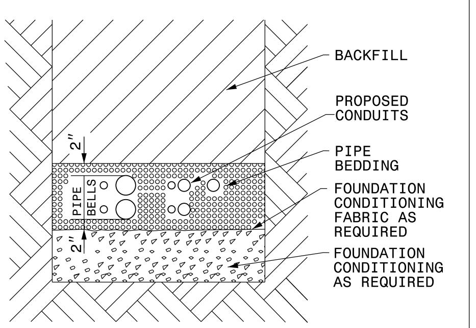
PLACE FOUNDATION CONDITIONING MATERIAL BELOW BEDDING IF REQUIRED, AS DIRECTED BY ENGINEER. PIPE BEDDED IN SELECT MATERIAL, CLASS II (TYPE 1) OR CLASS III. TRENCH BACKFILLED IN LOOSE 6" LAYERS COMPACTED TO TOP OF TRENCH USING LOCAL EXCAVATED MATERIAL IF APPROVED BY THE ENGINEER, OR SELECT MATERIAL. ALL MATERIAL SHALL BE FREE OF ROCKS, FOREIGN MATERIAL, AND FROZEN EARTH. COMPACTION SHALL BE TO APPROXIMATELY 95% DENSITY IN ACCORDANCE WITH AASHTO T-99 AS MODIFIED BY THE DEPARTMENT OF TRANSPORTATION.
