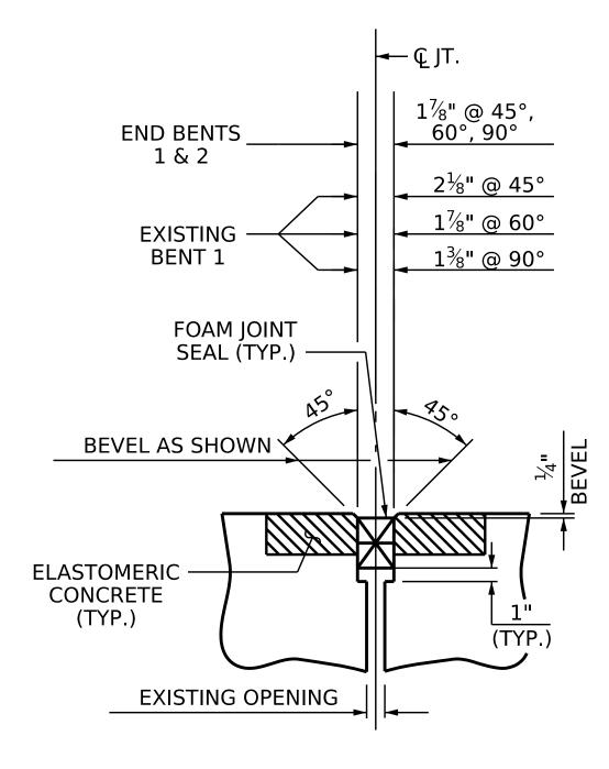
PROPOSED JOINT SEAL DETAIL
