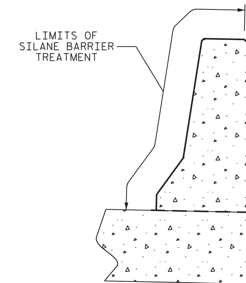
SILANE BARRIER RAIL TREATMENT
