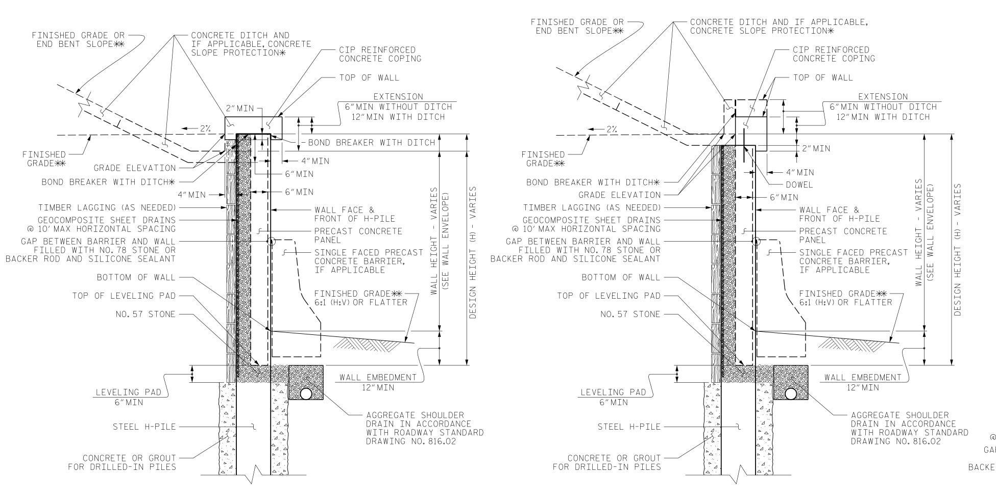
SOLDIER PILE WALL WITH PRECAST PANEL - TYPICAL SECTIONS
