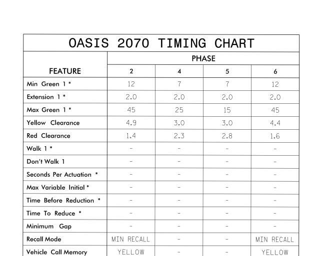
\* These values may be field adjusted. Do not adjust Min Green and Extension times for phases 2 and 6 lower than what is shown. Min Green for all other phases should not be lower than 4 seconds.
