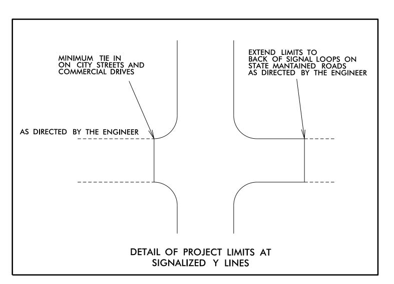
ALL UNPAVED S.R. ROADS TO BE RESURFACED 50' FROM EDGE OF PAVEMENT OF MAIN PROJECT. ALL PAVED S.R. ROADS TO BE RESURFACED TO THE ENDS OF THE RADII, OR AS DIRECTED BY THE ENGINEER. EDGES, PAVEMENT WIDENING, INTERSECTIONS AND BRIDGE FLARES ARE INCLUDED IN THE TABLE OF QUANTITIES. BRIDGES TO BE RESURFACED AT LOCATIONS AND TO DEPTH AS DIRECTED BY THE ENGINEER.
