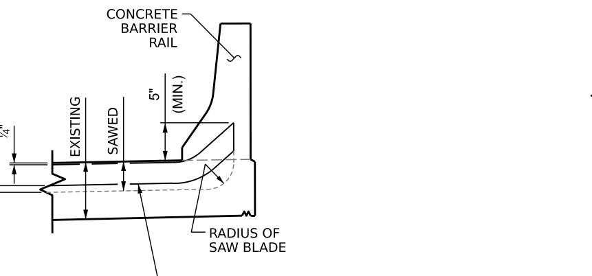
PROPOSED JOINT PRIOR TO SAWING
