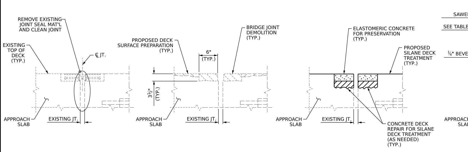
SAWED OPENING FOR JOINT SEE TABLE FOR JOINT OPENINGS 1/4" BEVEL AS SHOWN SEE DETAIL 'A' APPROACH EXISTING JT. **FOAM JOINT** SEAL (TYP.)
