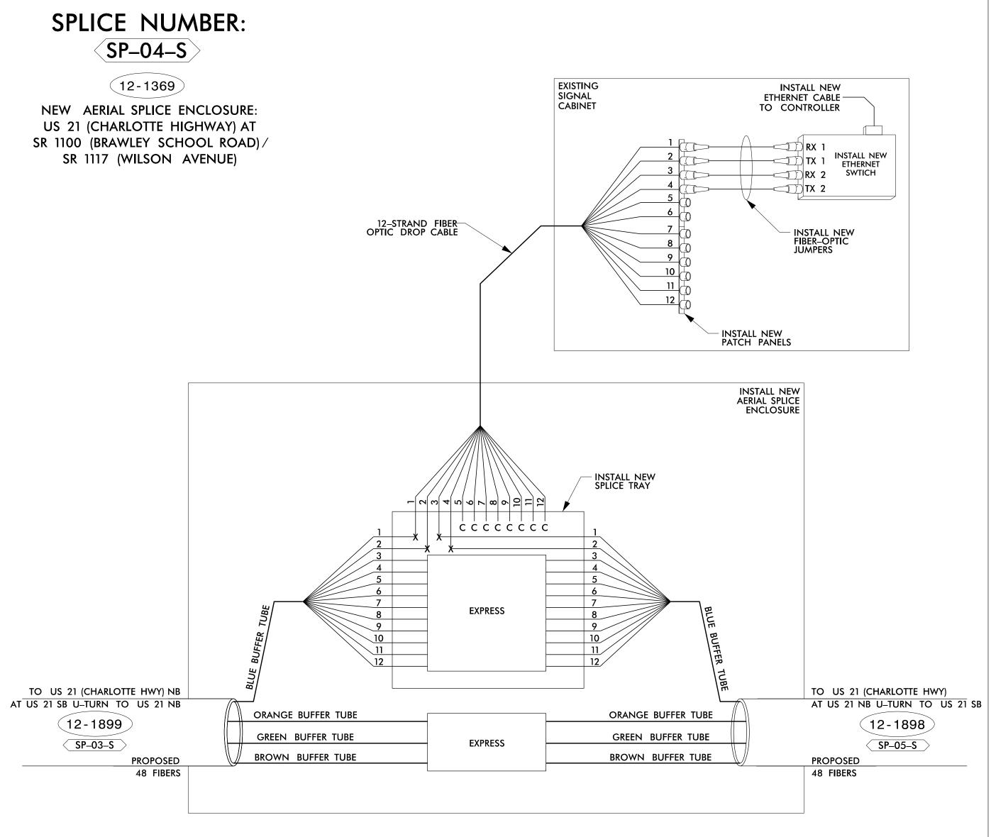
**LEGEND** COLOR CODE TIA/EIA 598-B EXISTING FUSION SPLICE INDIVIDUAL FIBER TO REMAIN (9) YELLOW X = FUSION SPLICE INDIVIDUAL FIBER (10) VIOLET C = CAP AND SEALEXPRESS ENTIRE BUFFER TUBE/FIBERS THROUGH WITHOUT CUTTING (12) AQUA **EXPRESS**
