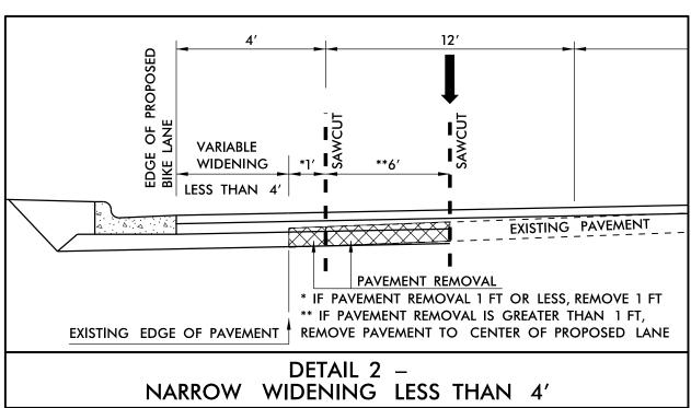
NOTE: ASSUMING MINIMAL WIDTH TO OBTAIN COMPACTION IS 5' AND THE DESIRE TO KEEP THE SAWCUT OUT OF THE PROPOSED WHEELPATH
