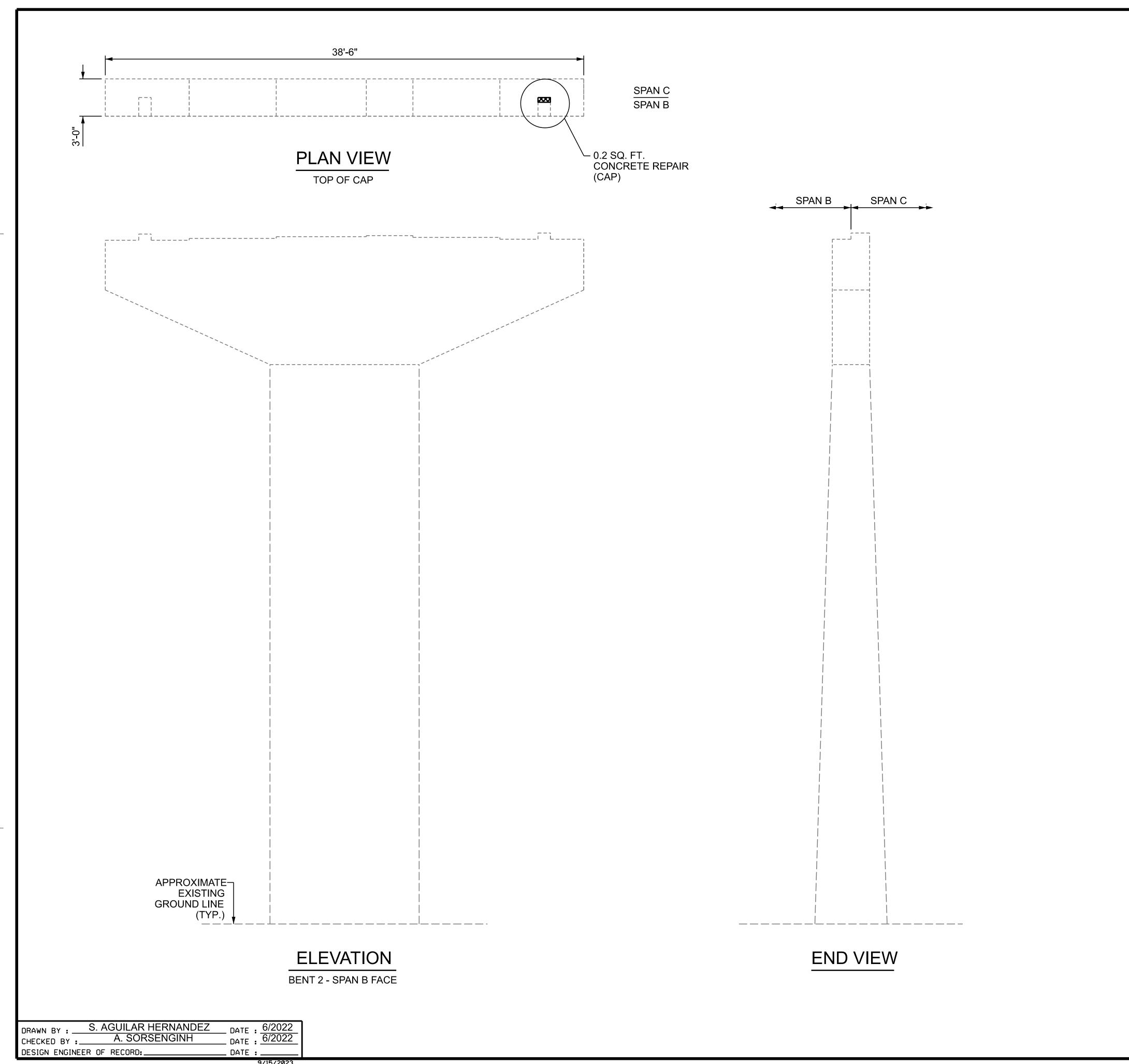
AS-BUILT REPAIR QUANTITY TABLE QUANTITIES BENT 2 - SPAN B FACE **ESTIMATE** ACTUAL AREA VOLUME AREA VOLUME SHOTCRETE REPAIRS SF CF CAP 0 0 COLUMN 0 AREA SF VOLUME AREA SF VOLUME CONCRETE REPAIRS 0.2 0.1 COLUMN 0 0 LINEAR LINEAR **EPOXY RESIN INJECTION** FT CAP 0 0 COLUMN AREA AREA **EPOXY COATING** TOP OF BENT CAP 102.0
