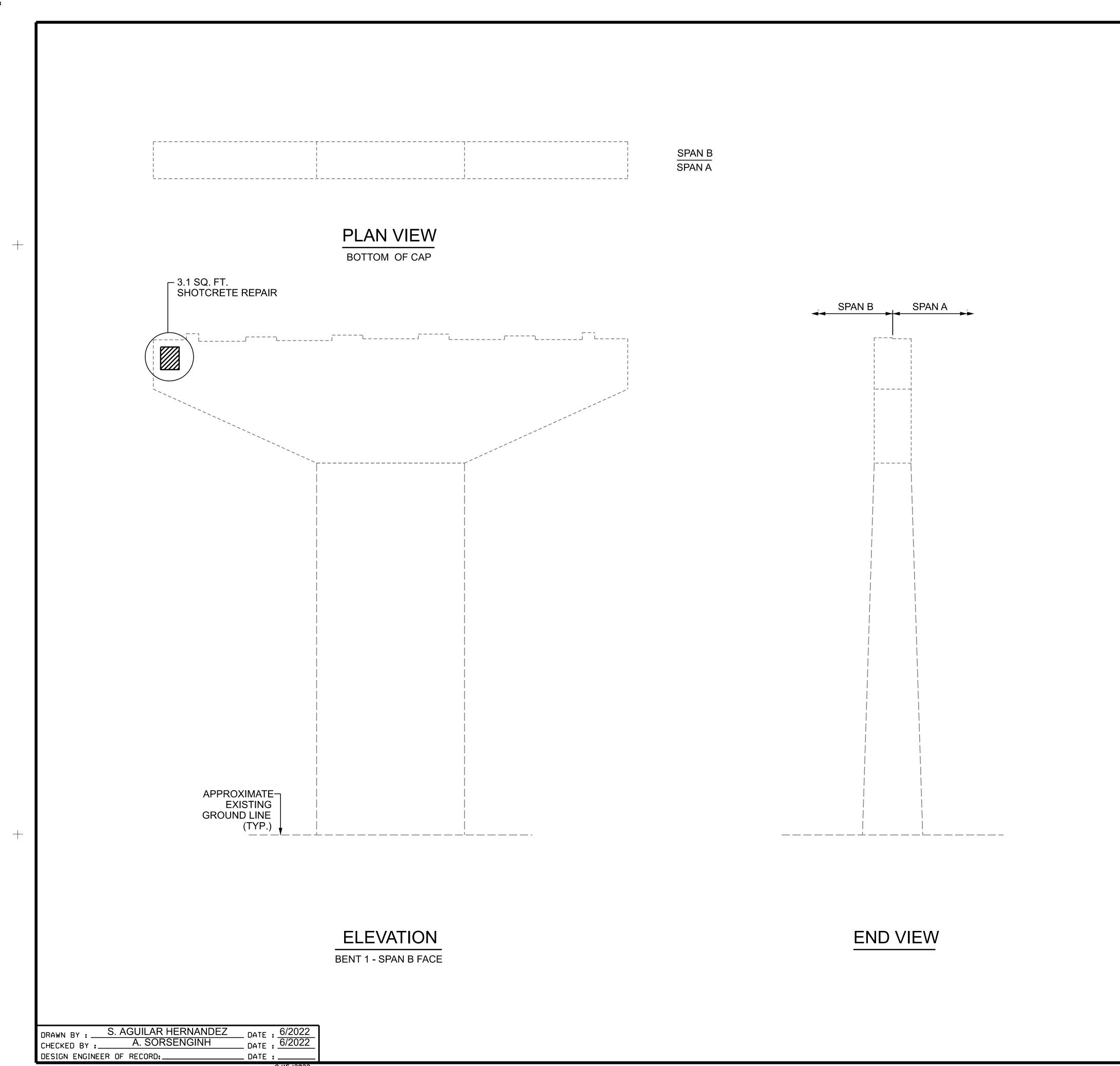
AS-BUILT REPAIR QUANTITY TABLE QUANTITIES BENT 1 - SPAN B FACE **ESTIMATE** ACTUAL AREA AREA VOLUME VOLUME SHOTCRETE REPAIRS SF CAP 3.1 1.6 COLUMN 0 0 AREA SF VOLUME AREA SF VOLUME CONCRETE REPAIRS 0 COLUMN 0 0 LINEAR LINEAR **EPOXY RESIN INJECTION** FT CAP 0 COLUMN
