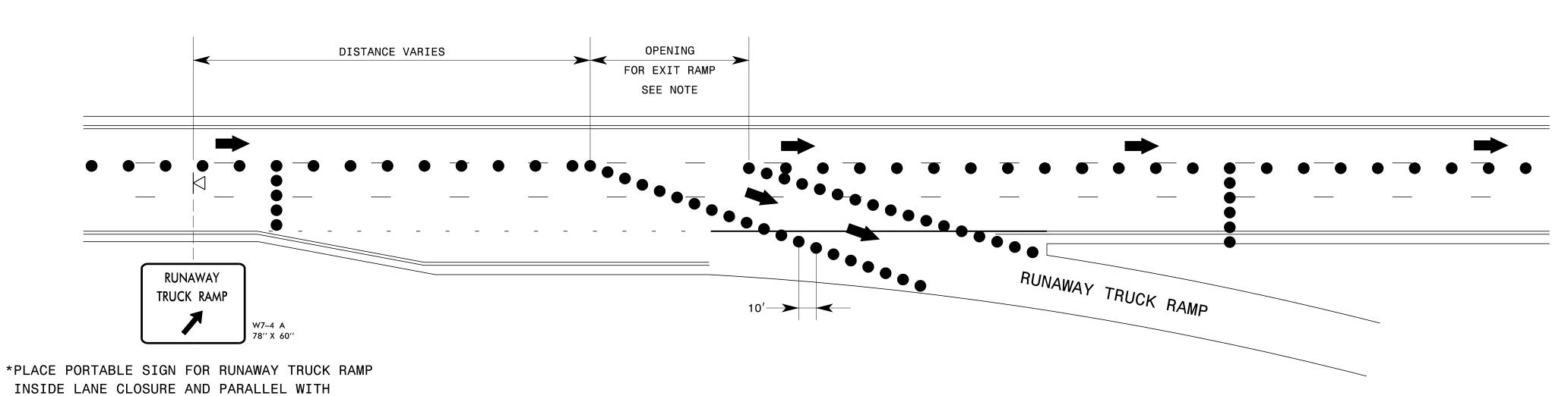
NOTES: MAINTAIN A MINIMUM 250' OPENING FOR RUNAWAY TRUCK EXIT RAMPS OR AS DIRECTED BY THE ENGINEER. CLOSE RAMPS WHEN ACTIVE WORK AREAS ARE WITHIN 500' OF EACH LOCATION. INSTALL TEMPORARY RUNAWAY TRUCK RAMP SETUP WHEN RESURFACING CENTER LANE OR OUTSIDE LANE WITHIN
