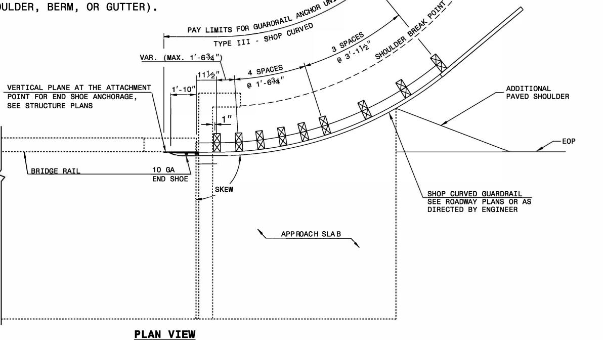
GUARDRAIL ANCHOR UNIT, TYPE III - SHOP CURVED FOR ATTACHMENT TO RAIL ON BRIDGE
