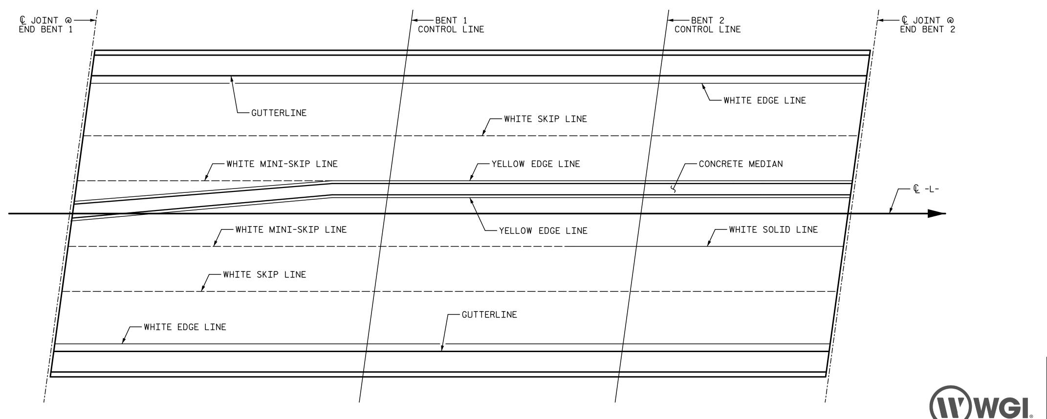
PAVEMENT MARKING ALIGNMENT
