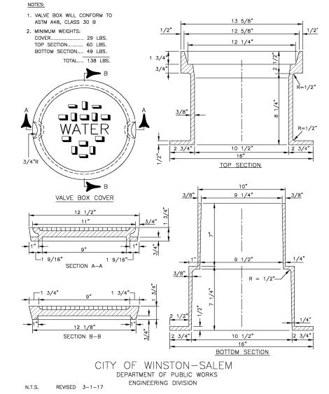
CAST IRON VALVE BOX UC-3B NOT TO SCALE
