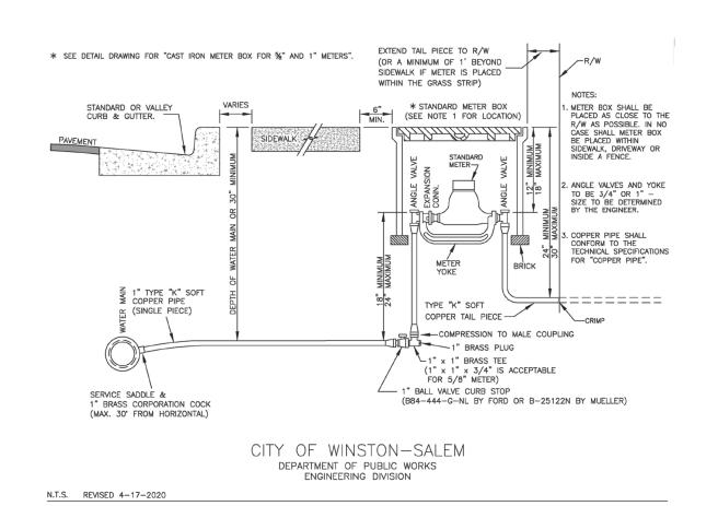
1" WATER CONNECTION (WITH CURB & GUTTER/SINGLE FAMILY) UC-3B NOT TO SCALE
