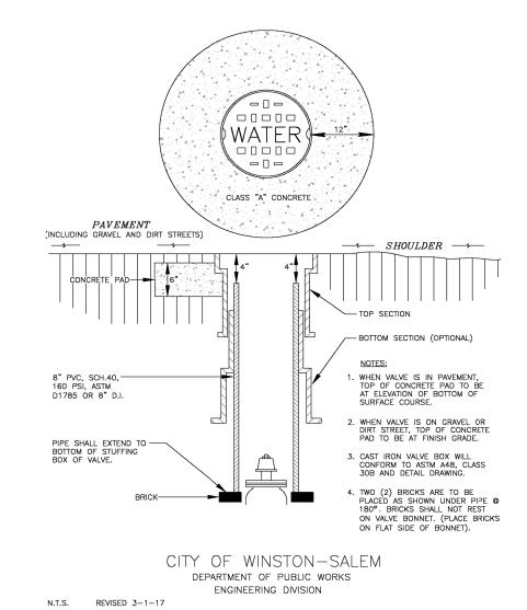
VALVE BOX INSTALLATION \UC-3B / NOT TO SCALE
