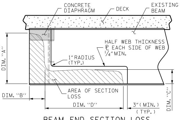
BEAM END SECTION LOSS AND PLATING REPAIR
