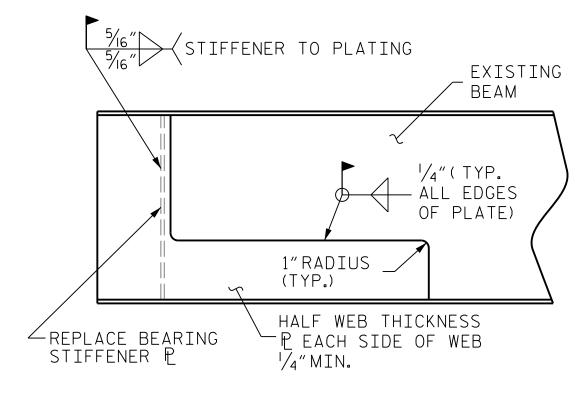
BEAM END PLATING REPAIR
