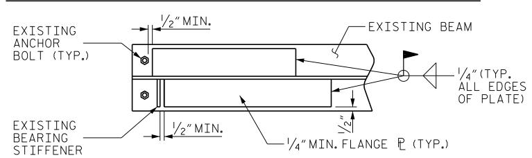
FLANGE PLATING REPAIR TYPE ''D''
