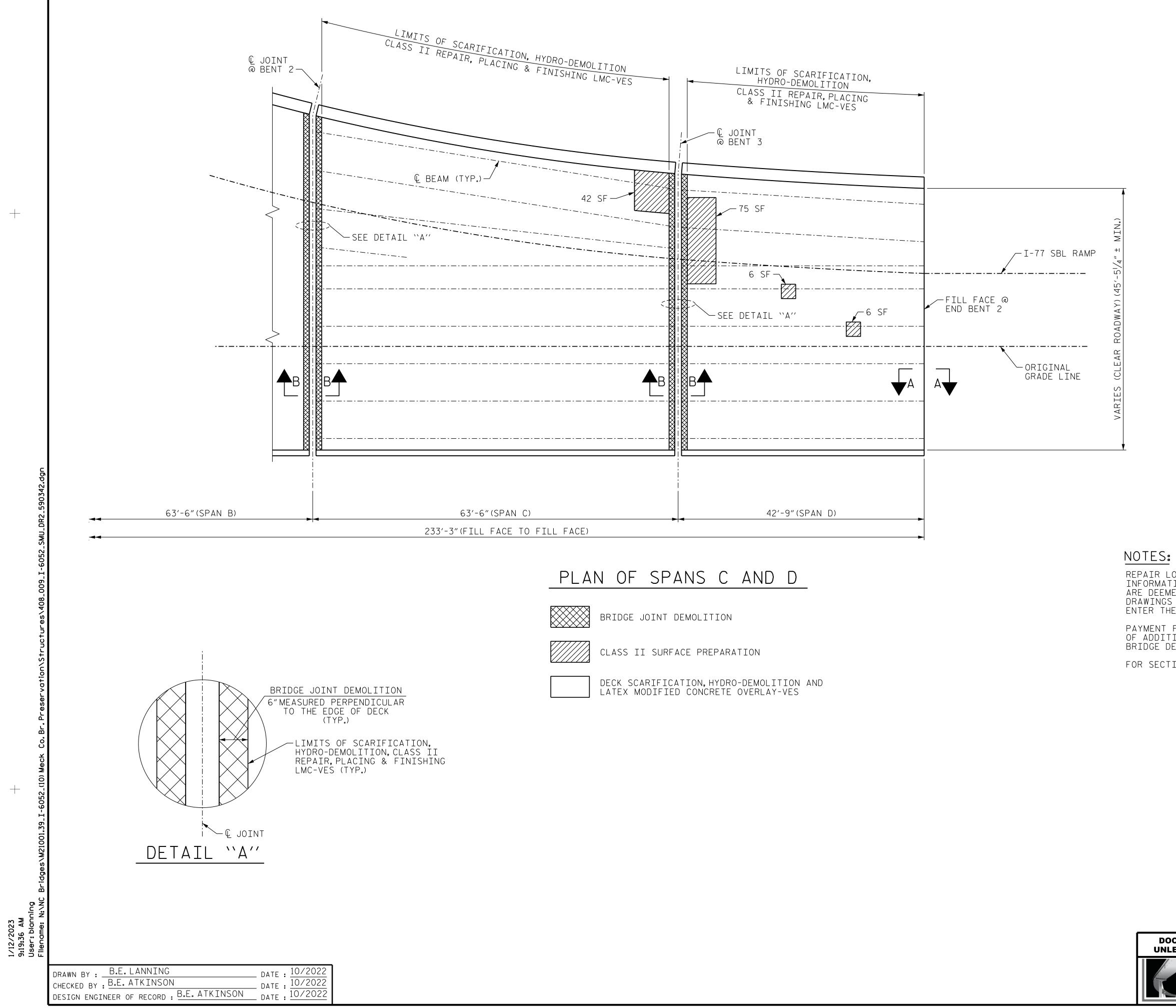
REPAIR LOCATIONS AND ESTIMATE OF QUANTITIES ARE BASED ON THE BEST INFORMATION AVAILABLE. IF ADDITIONAL REPAIRS NOT SHOWN ON THE DRAWINGS ARE DEEMED NECESSARY BY THE ENGINEER, THE ENGINEER WILL NOTE ON THE DRAWINGS THE APPROXIMATE LOCATIONS AND DESCRIPTION OF THE REPAIRS AND ENTER THE ACTUAL QUANTITIES INTO THE AS-BUILT REPAIR QUANTITY TABLE.
