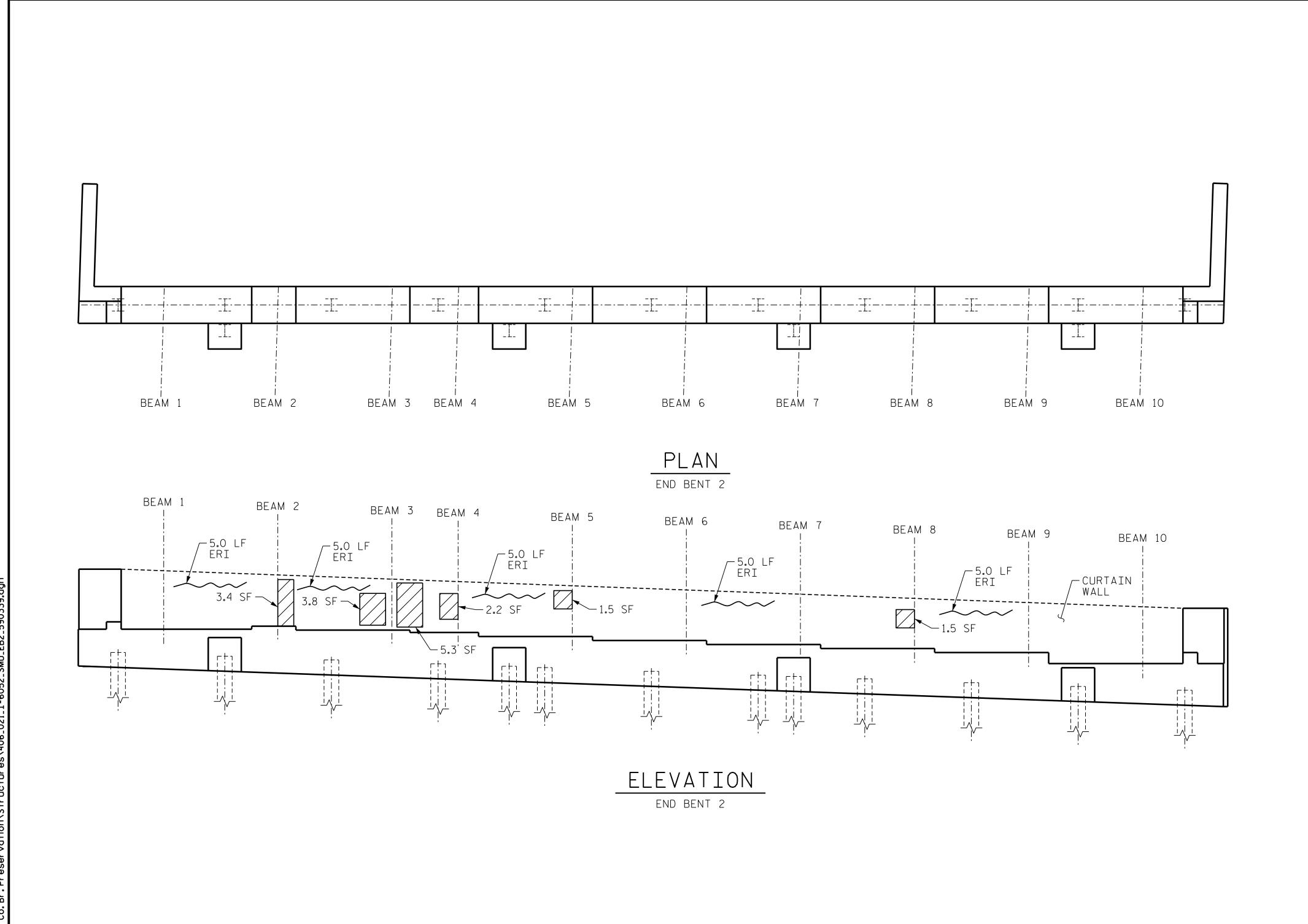
AS-BUILT REPAIR QUANTITY TABLE QUANTITIES END BENT 2 ESTIMATE ACTUAL AREA VOLUME VOLUME SHOTCRETE REPAIRS CF CF CAP (VERTICAL FACE) 0.0 0.0 CAP (HORIZONTAL FACE) 0.0 0.0 CURTAIN WALL 17.7 8.9 VOLUME | AREA VOLUME CONCRETE REPAIRS CAP 0.0 0.0 EPOXY RESIN INJECTION LIN.FT. LIN.FT. 0.0 25.0 CURTAIN WALL AREA AREA EPOXY COATING SF SF TOP OF CAP 116.8
