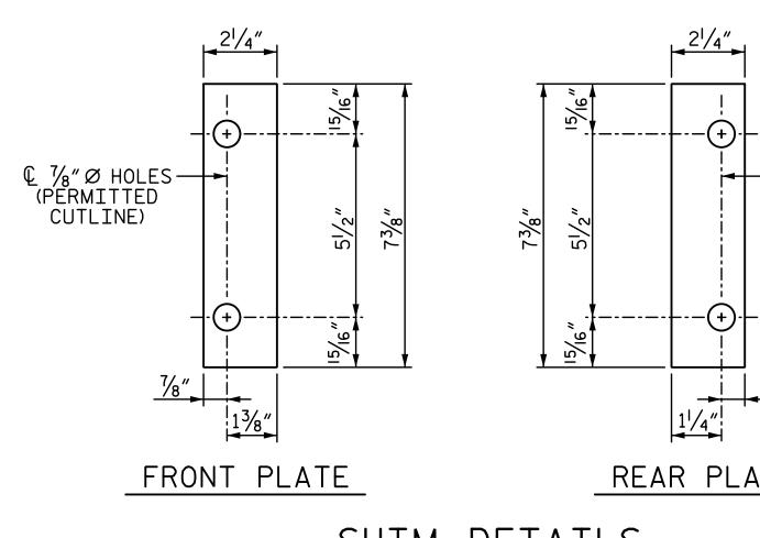
SHIM DETAILS NOTE: SHIMS MAY BE CUT ALONG PERMITTED CUTLINE OR SLOTTED TO EDGE OF PLATE TO FACILITATE PLAEMENT.
