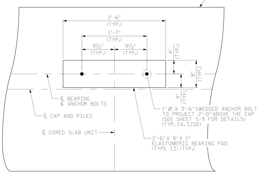
DETAIL ``A'' END BENT NO.2.SHOWN,END BENT NO.1SIMILAR BUT OPPOSITE HAND. DIMENSIONS ARE TYPICAL FOR EACH GIRDER. PILES NOT SHOWN FOR CLARITY.
