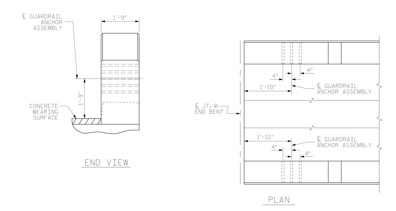
LOCATION OF GUARDRAIL ANCHOR AT END POST
