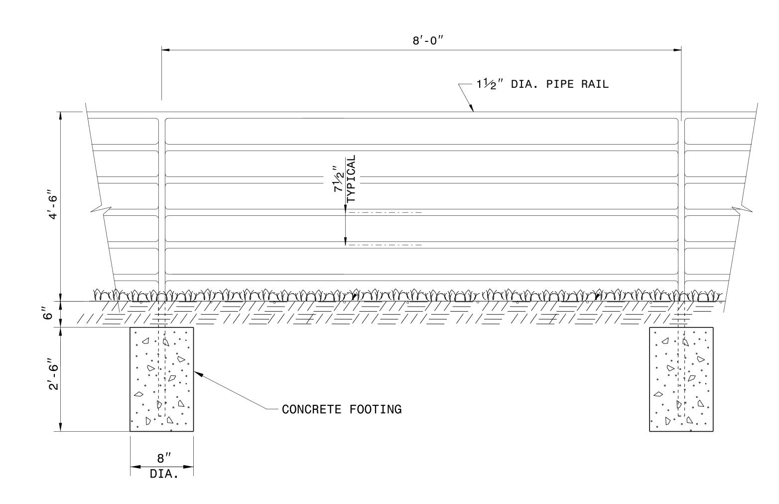
**ELEVATION OF HANDRAIL**
