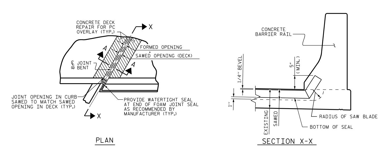
JOINT SEAL TO BE CUT, HEAT WELDED AND TURNED UP PARALLEL TO SLOPED FACE OF THE SIDEWALK.
