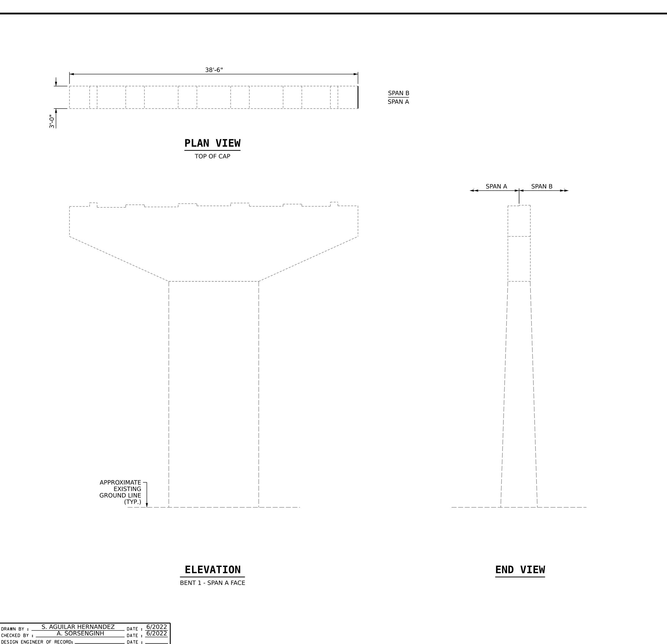
AS-BUILT REPAIR QUANTITY TABLE QUANTITIES BENT 1 - SPAN A FACE ACTUAL **ESTIMATE** AREA AREA VOLUME VOLUME SHOTCRETE REPAIRS SF CAP 0 0 COLUMN 0 VOLUME AREA SF AREA SF VOLUME CONCRETE REPAIRS 0 COLUMN 0 0 LINEAR LINEAR **EPOXY RESIN INJECTION** FΤ COLUMN AREA AREA EPOXY COATING TOP OF BENT CAP 102.0
