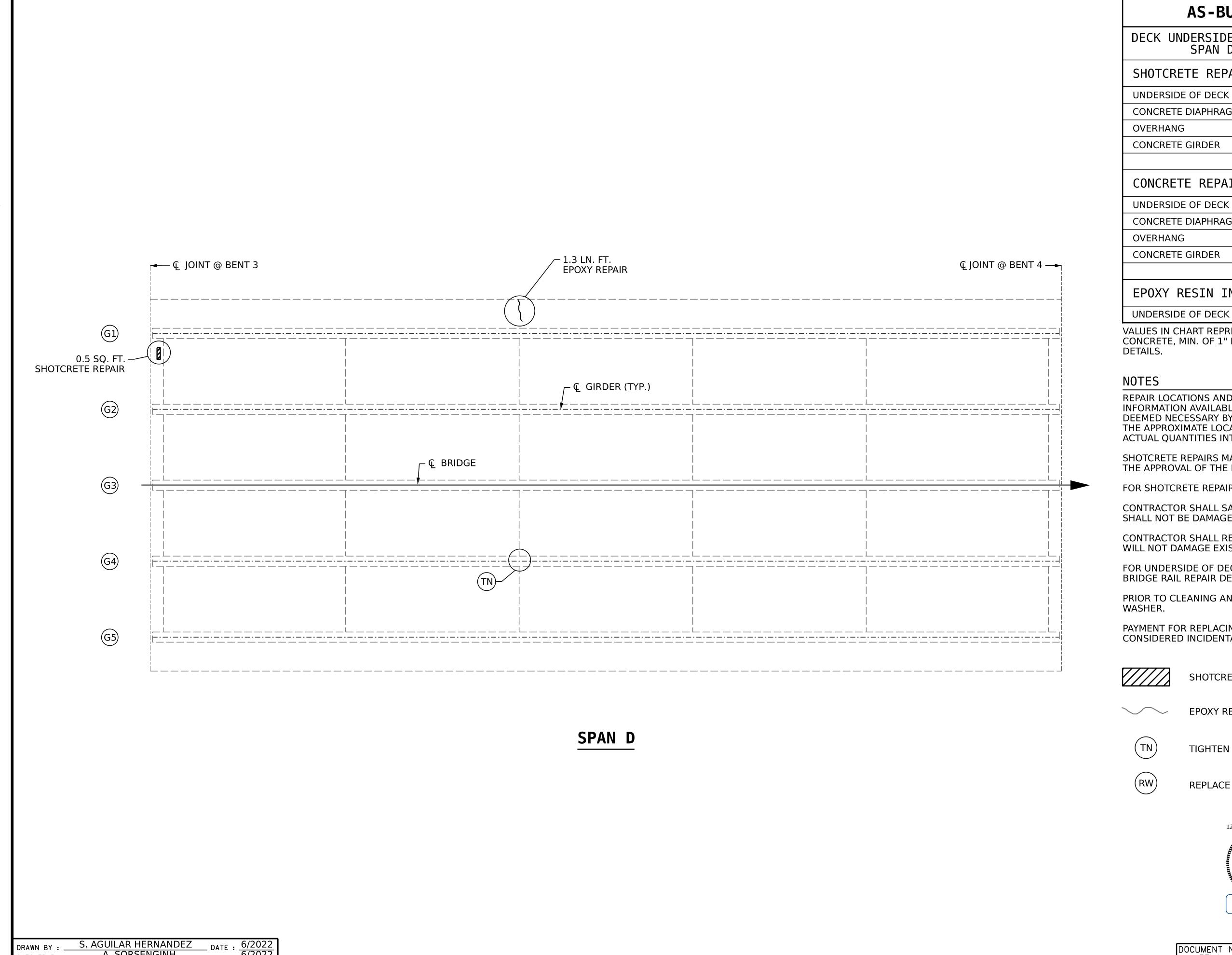
AS-BUILT REPAIR QUANTITY TABLE DECK UNDERSIDE REPAIRS SPAN D QUANTITIES **ESTIMATE** ACTUAL VOLUME AREA VOLUME AREA SHOTCRETE REPAIRS SF UNDERSIDE OF DECK 0 CONCRETE DIAPHRAGM 0.5 0.3 OVERHANG 0 CONCRETE GIRDER VOLUME VOLUME AREA CONCRETE REPAIRS CF UNDERSIDE OF DECK 0 CONCRETE DIAPHRAGM CONCRETE GIRDER 0 LINEAR LINEAR EPOXY RESIN INJECTION FT
