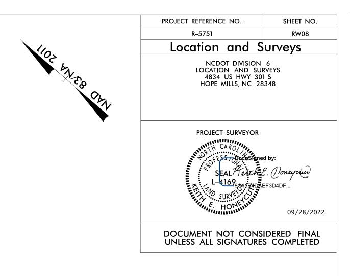
I, Keith E. Honeycutt, PLS., certify that the right of way and permanent easement monumentation for this project shown herein was completed under my direct and responsible charge from an actual survey made under my supervision; that all horizontal closures had a minimum ratio of precision of 1:10,000 (Class A). Field work was performed in March 2022, and all coordinates are based on NAD83/2011; That this survey was performed to meet the requirements of 21NCAC 56.1600 as applicable.
