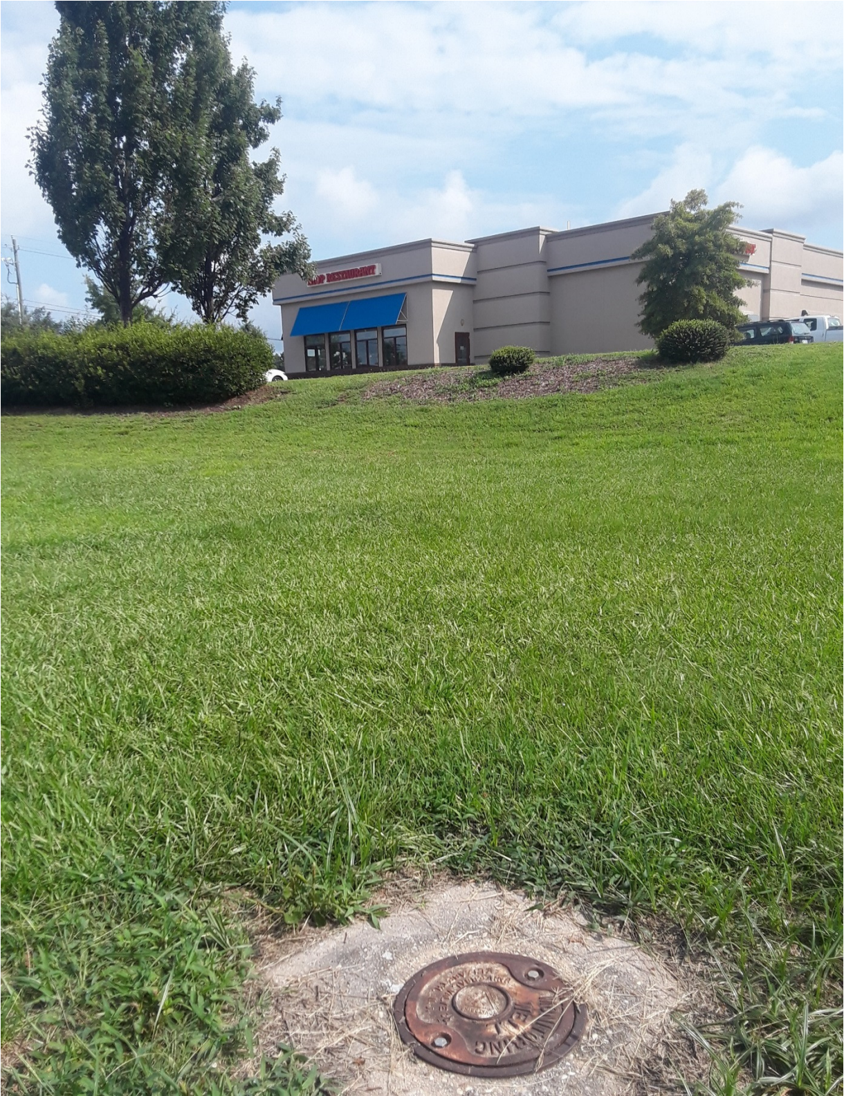
Photo 3 – A view of the two-inch diameter monitoring well (abandoned) in the railroad right of way.
