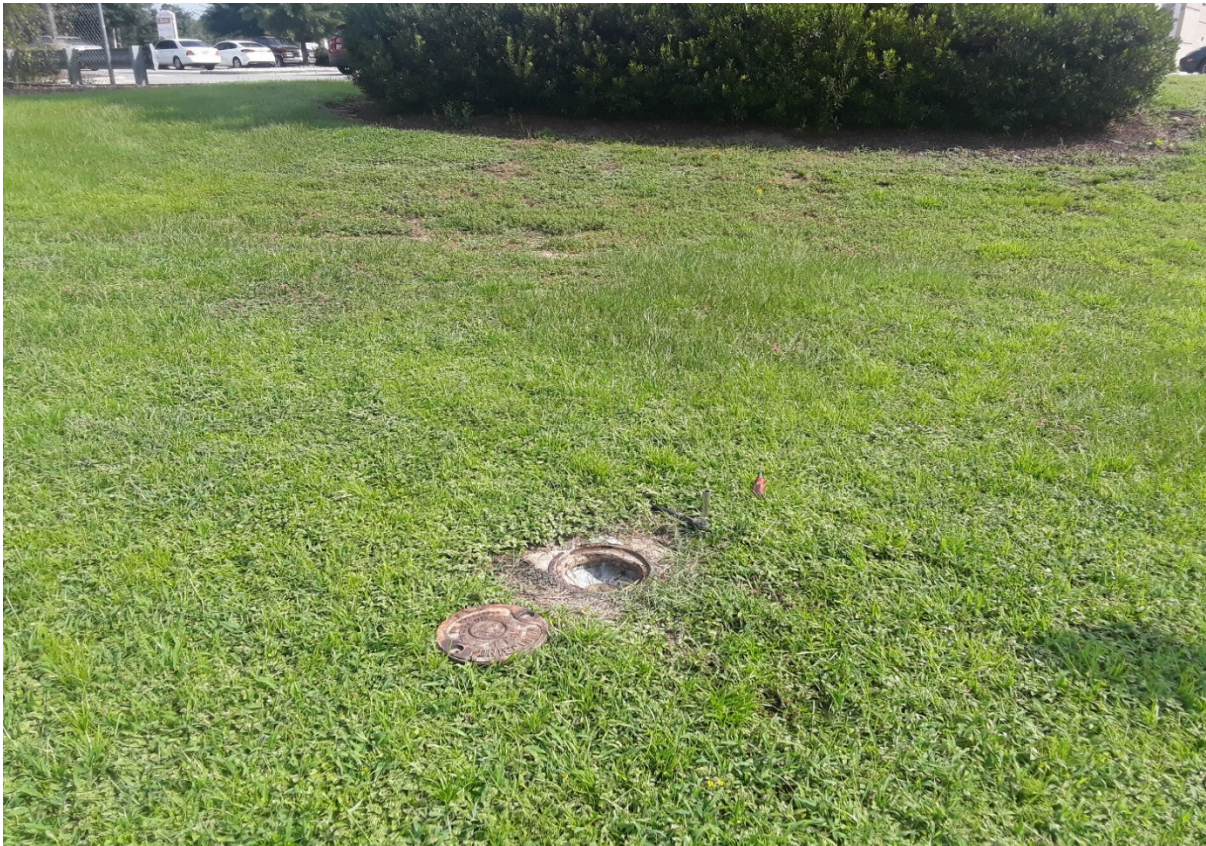
Photo 2 – A view of the four-inch diameter monitoring well (abandoned) in the railroad right of way.
