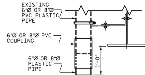
**6" OR 8" PIPE DRAIN EXTENSION DETAIL**
