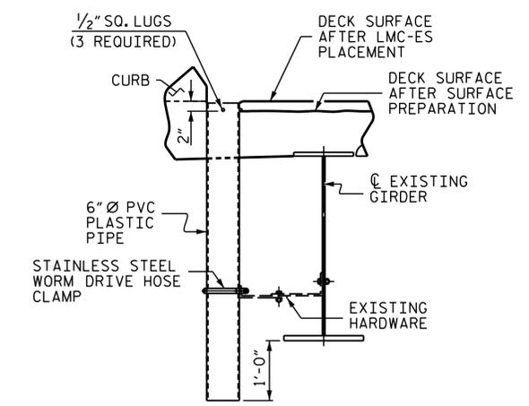
**PIPE DRAIN REPLACEMENT DETAIL**
