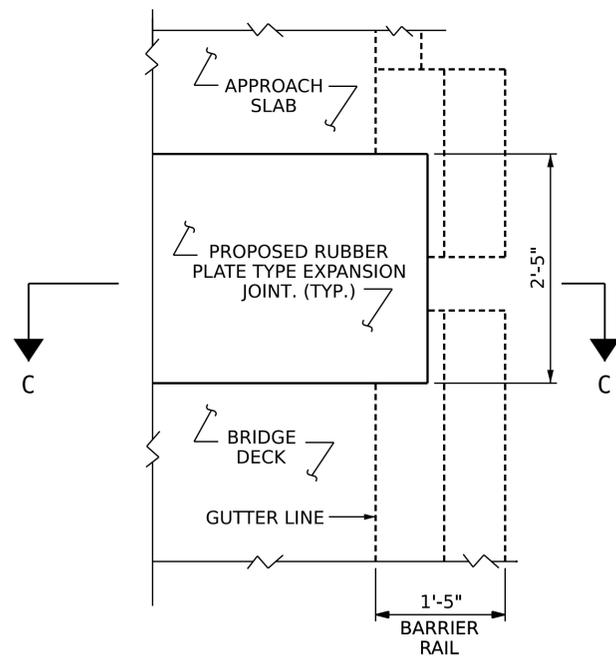
PLAN OF PROPOSED EXPANSION JOINT SEAL
