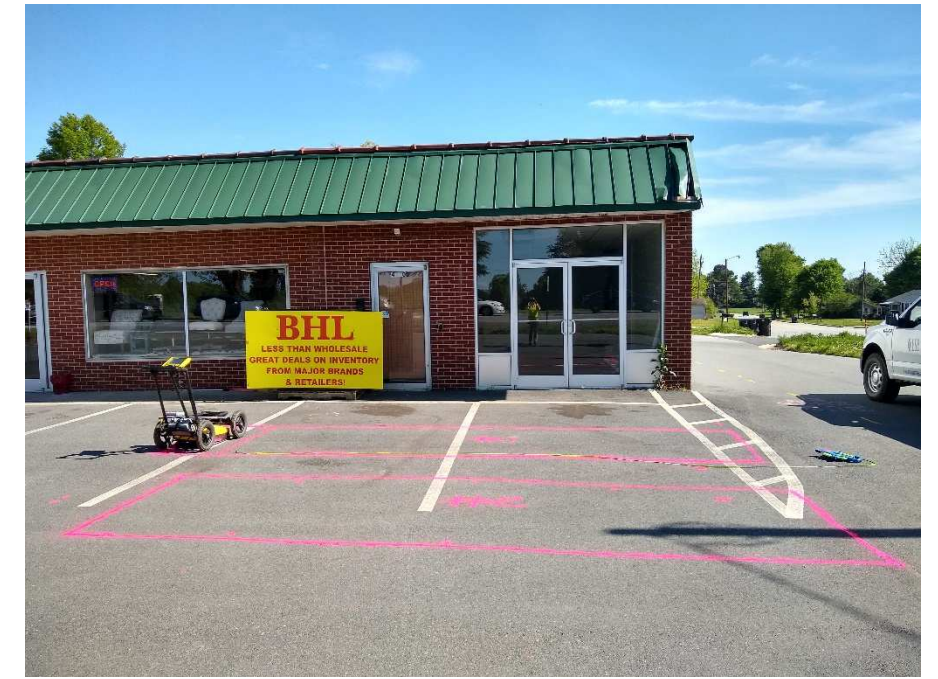
C. Photograph of marked location of two probable USTs in the northwest part of the site, facing south.
