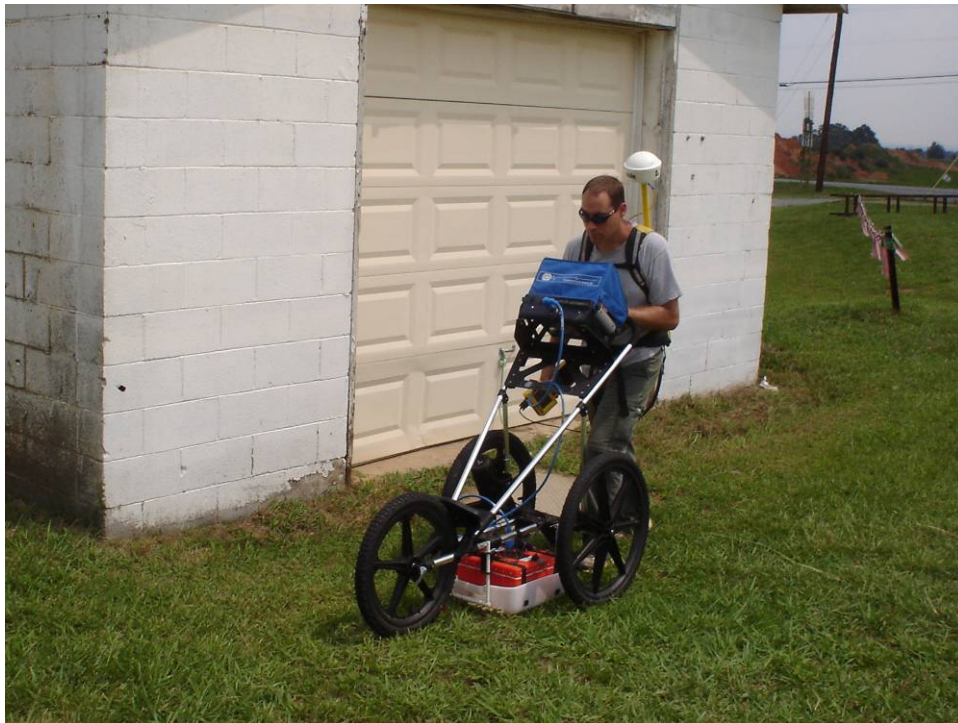
GSSI SIR-3000 Ground-Penetrating Radar with 400 MHz Antenna
