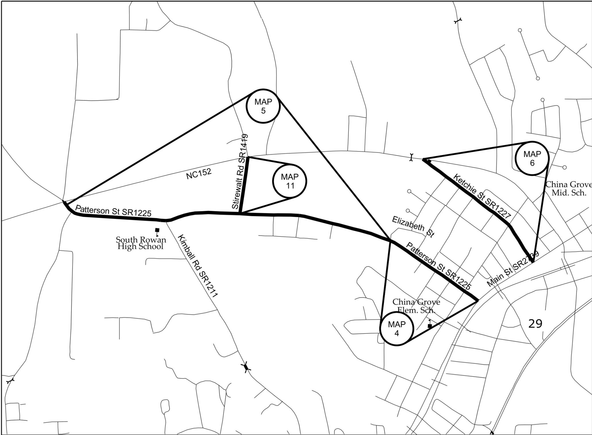
Map 4 Patterson St SR1225 From Main St SR2739 to end of curb approx. 180' past Elizabeth St Mill 2" entire width to be flush with gutter Mill 0-11/2" 7' width along gutter Patching to be done by DOT forces Pave 11/2" S9.5B
