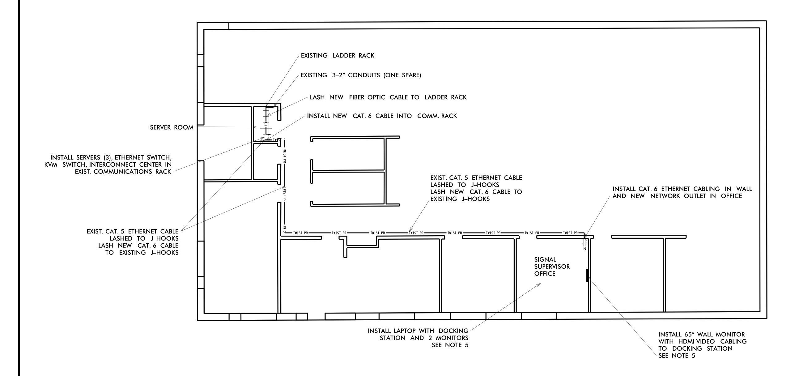
LEGEND PROPOSED ETHERNET CABLE PROPOSED FIBER-OPTIC CABLE PROPOSED NETWORK OUTLET
