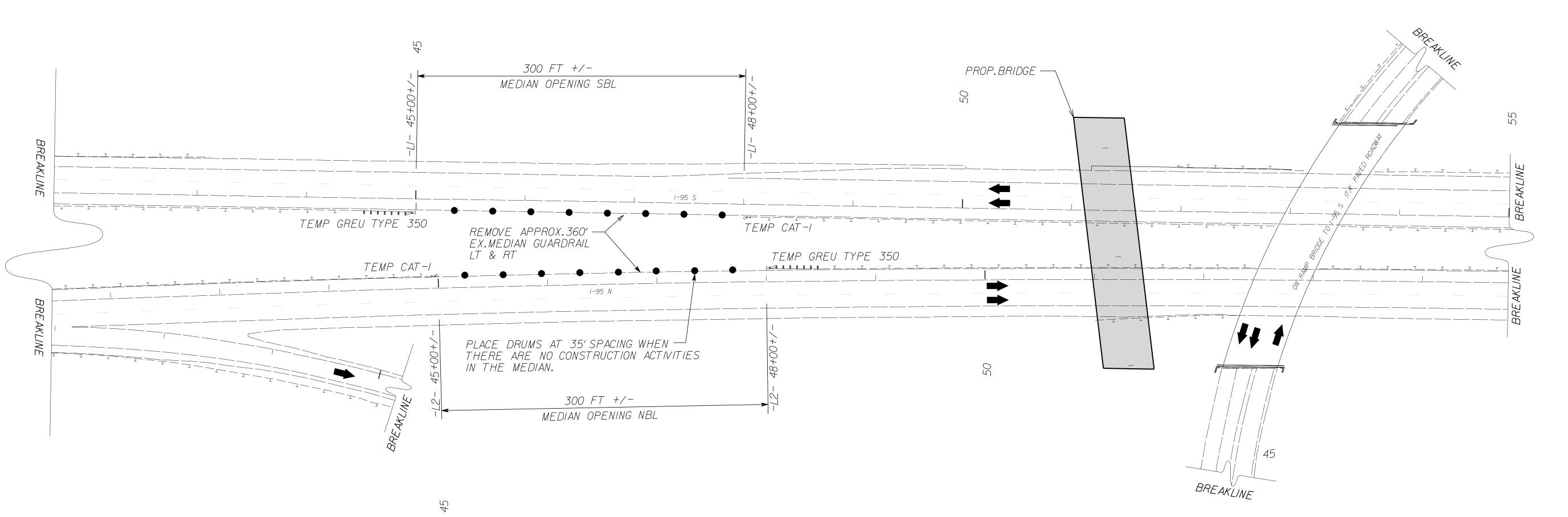
REPLACE MEDIAN GUARDRAIL WHEN CONTRACTOR ACCESS NO LONGER REQUIRED
