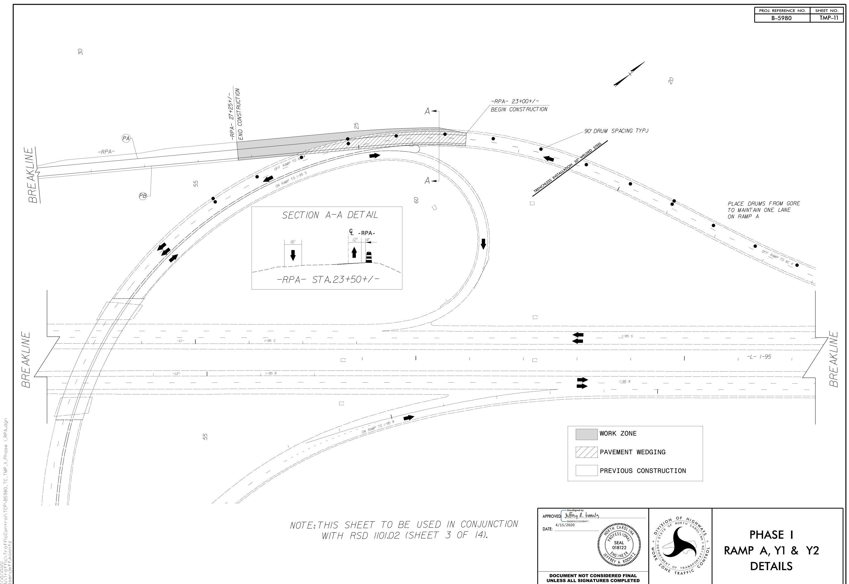
PROJ. REFERENCE NO. B-5980 TMP-12 LOCATE APPROX. 1/2 MILE IN ADVANCE OF DETOUR PLACE PAVEMENT MARKING ON EXISTING RAMP PAVEMENT IN FINAL PATTERN FOR SINGLE LANE (SEE PAVEMENT MARKING PLANS) ,45' DRUM SPACING (TYP.) *⊢2" OVERLAY* TEMPORARY TRAFFIC PATTERN FOR RAMP A AND SR 1544 (HALIFAX ROAD) APPROVED: Jeffry 1. 20047
