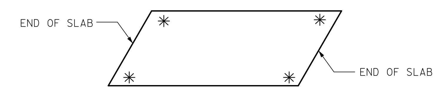
SKETCH SHOWING POINTS OF ATTACHMENTS
