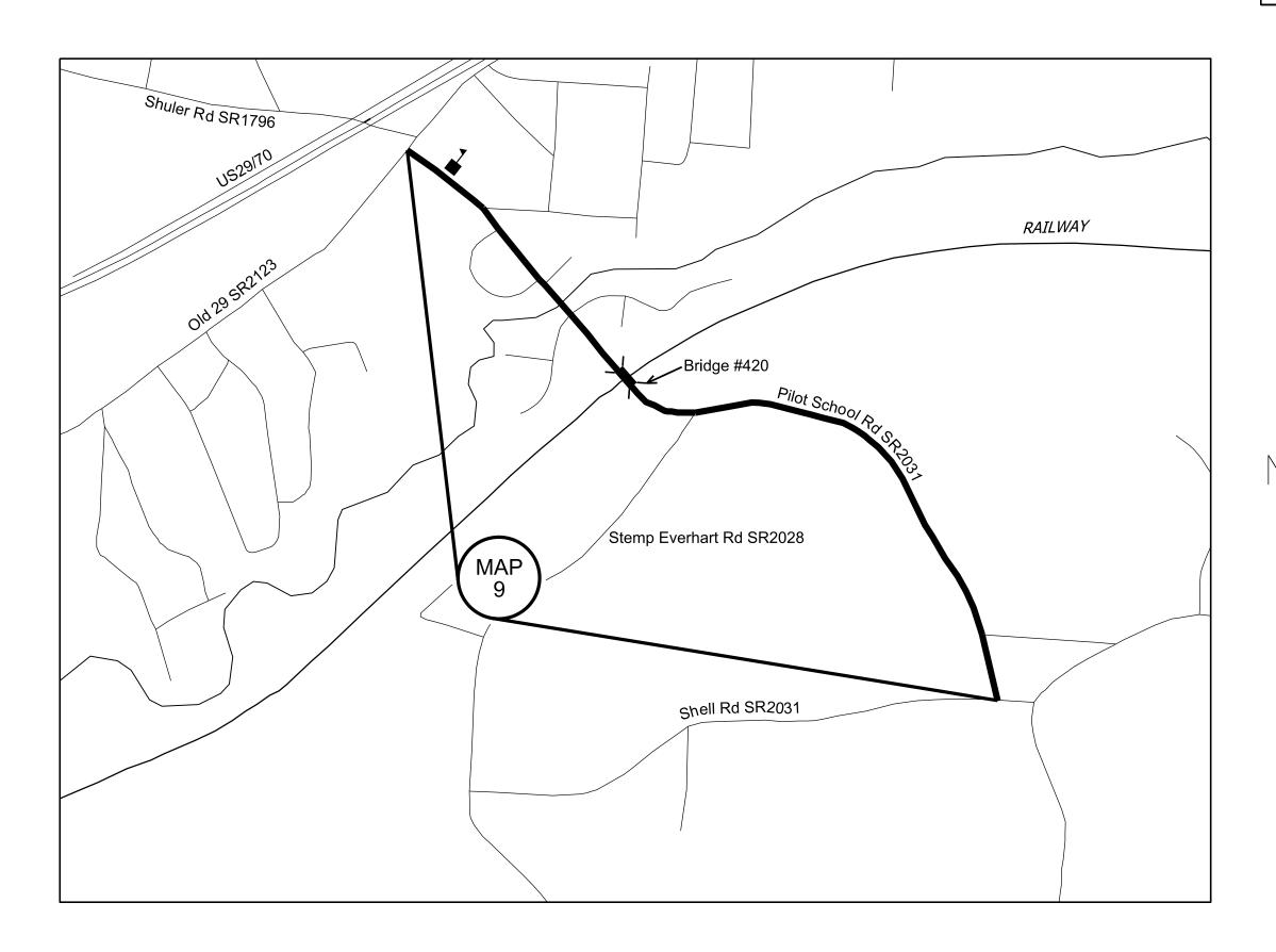
Map 9 Pilot School Rd SR2031 From Old 29 SR2123 to Shell Rd SR2031 Mill 0-1 1/2" incidental beginning, end,all SR intersections and at Bridge #420 Mill 0-1 1/2" at 7' width along curb and gutter Pave 1 1/2" S9.5B
