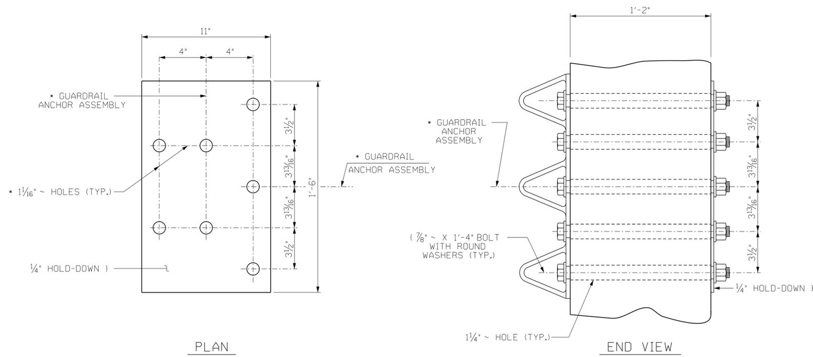
GUARDRAIL ANCHOR ASSEMBLY DETAILS
