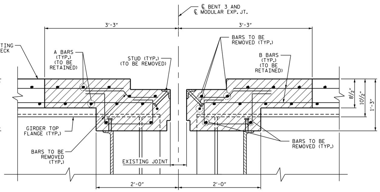
MODULAR EXPANSION JOINT DEMOLITION SECTION D-D
