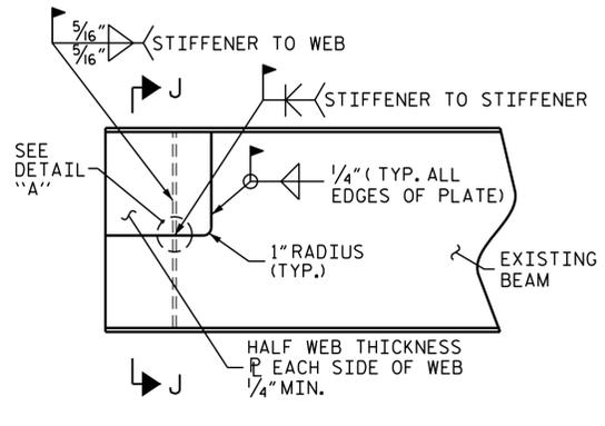
**BEAM END PLATING REPAIR**
