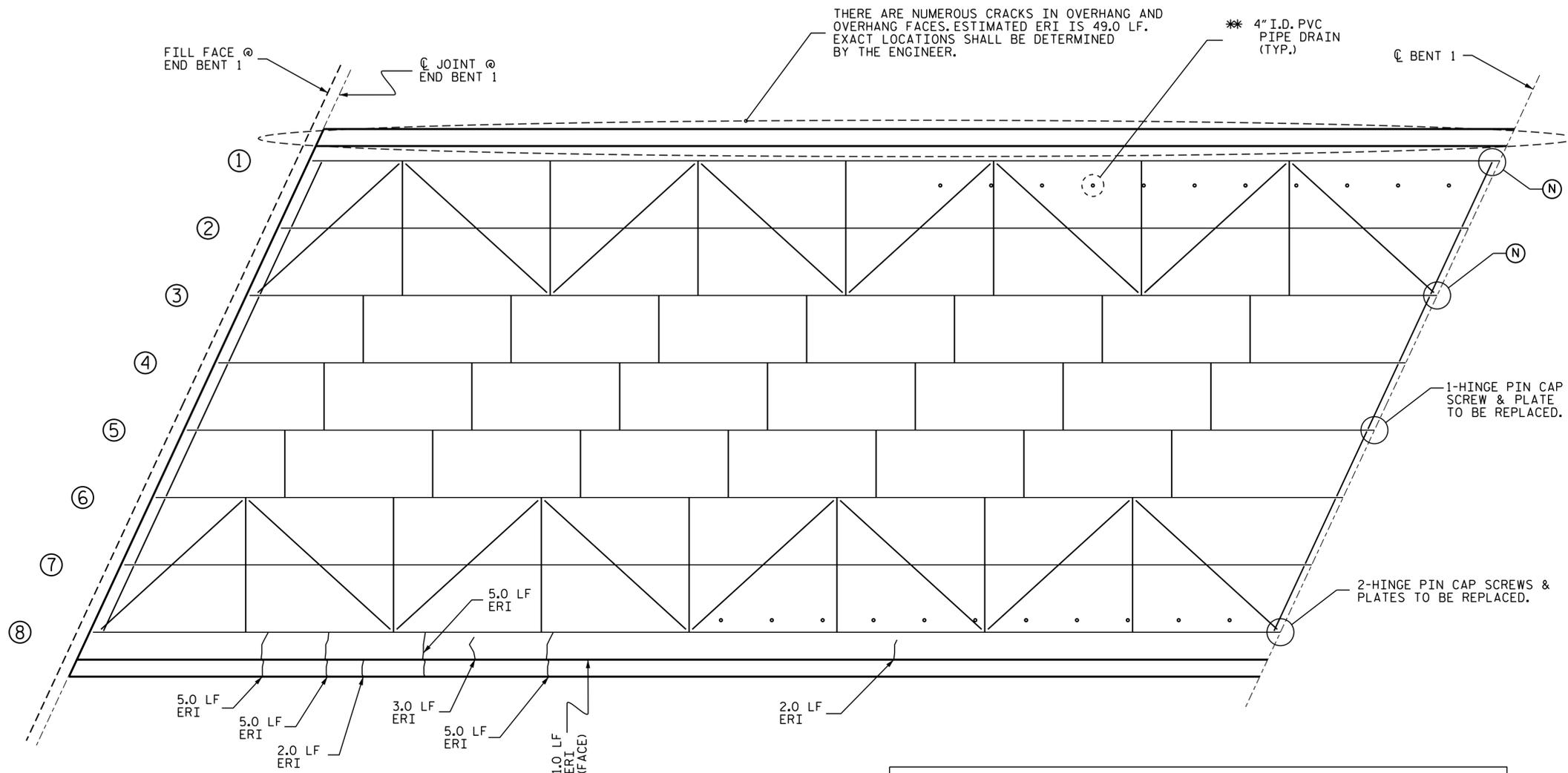
\*\* THE FIELD ENGINEER SHALL DETERMINE THE ACTUAL NUMBER OF REPAIR LOCATIONS. 4 LOCATIONS NOTED DURING FIELD EVALUATION. ESTIMATE QUANTITY, 1.1 CF OF SHOTCRETE EACH LOCATION ADDED TO "UNDERSIDE OF DECK" IN QUANTITY TABLE.
