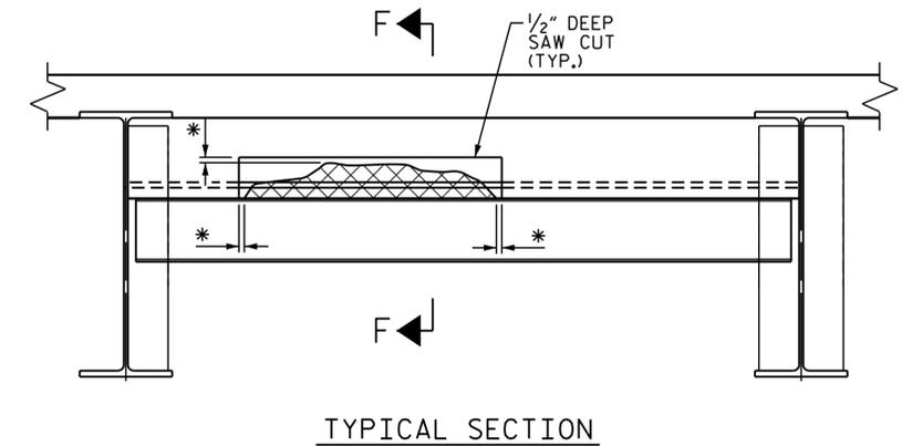
\* REMOVE CONCRETE UNTIL SOUND CONCRETE IS FOUND (2" MIN. CL.)
