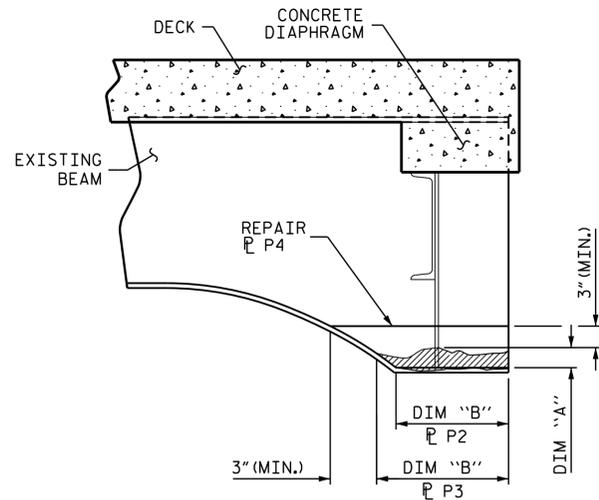
**BEAM END SECTION LOSS AND PLATING REPAIR**
