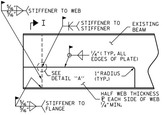
**BEAM END PLATING REPAIR**
