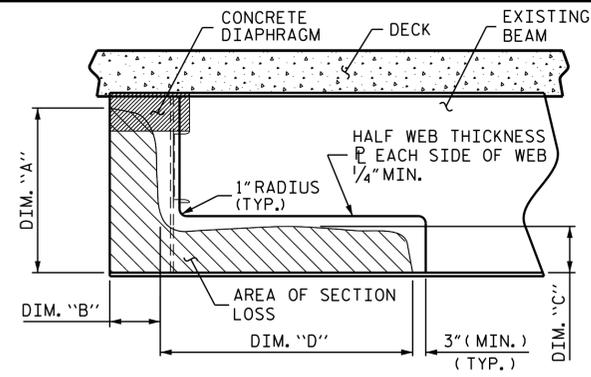
**BEAM END SECTION LOSS AND PLATING REPAIR**
