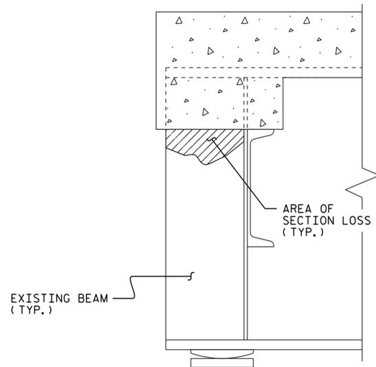
**BEAM END SECTION LOSS**
