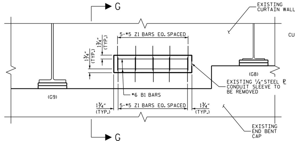
SEALING EXISTING 1/4" STEEL PIPE CONDUIT SLEEVE
