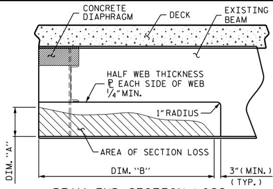
**BEAM END SECTION LOSS AND PLATING REPAIR**
