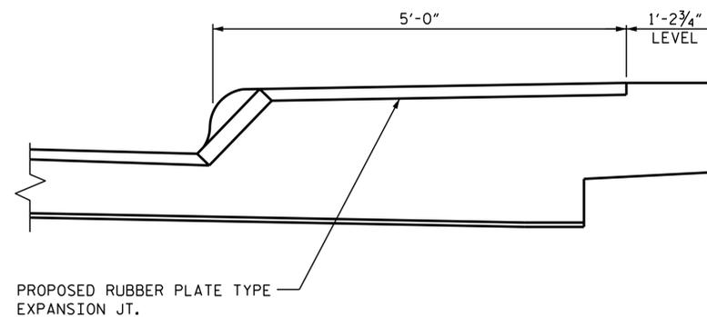
**MODULAR JOINT SEAL DETAILS THRU SIDEWALK**
