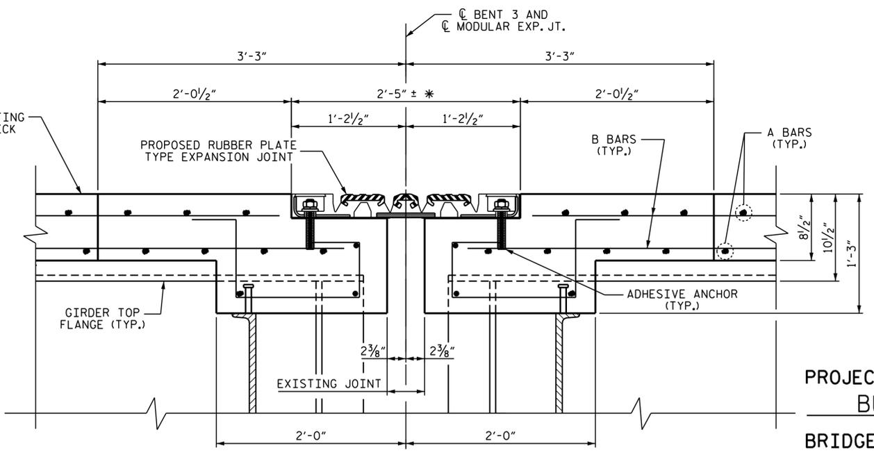
PROPOSED MODULAR EXPANSION JOINT REPAIR SECTION D-D
