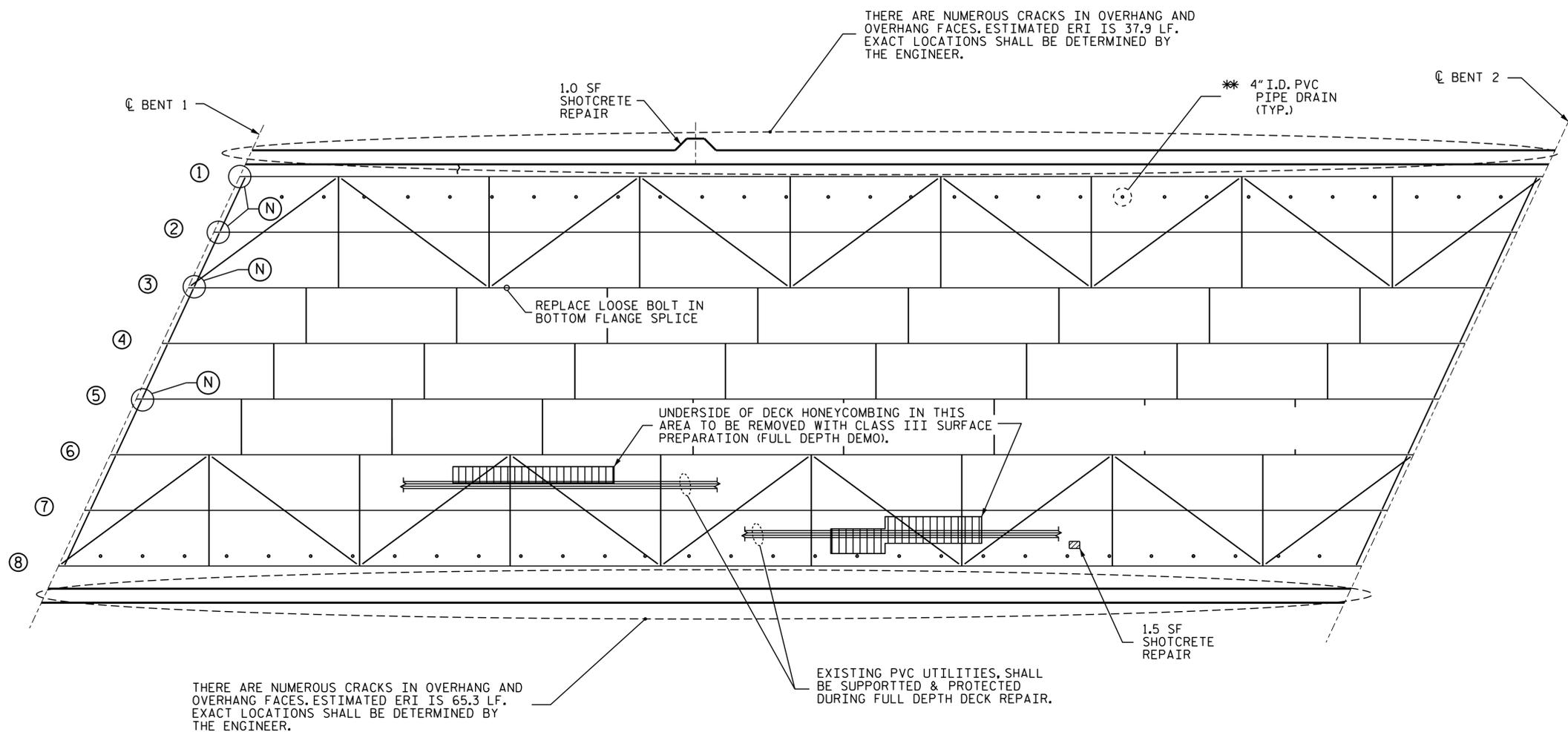
THERE ARE NUMEROUS CRACKS IN OVERHANG AND OVERHANG FACES. ESTIMATED ERI IS 65.3 LF. EXACT LOCATIONS SHALL BE DETERMINED BY THE ENGINEER.
