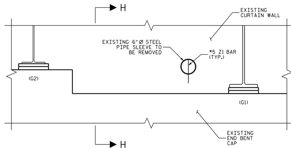
SEALING EXISTING 6" Ø STEEL PIPE SLEEVE
