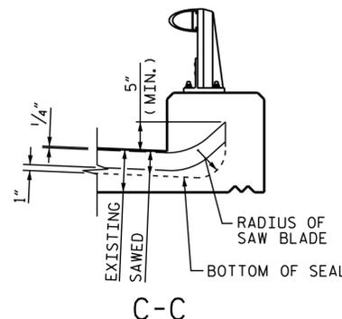
FOAM JOINT SEAL SHALL BE FACTORY FORMED OR CUT, HEAT WELDED AND TURNED UP PARALLEL TO FACE OF CURB.
