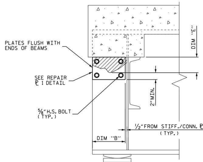
**BEAM END SECTION LOSS PLATING REPAIR**
