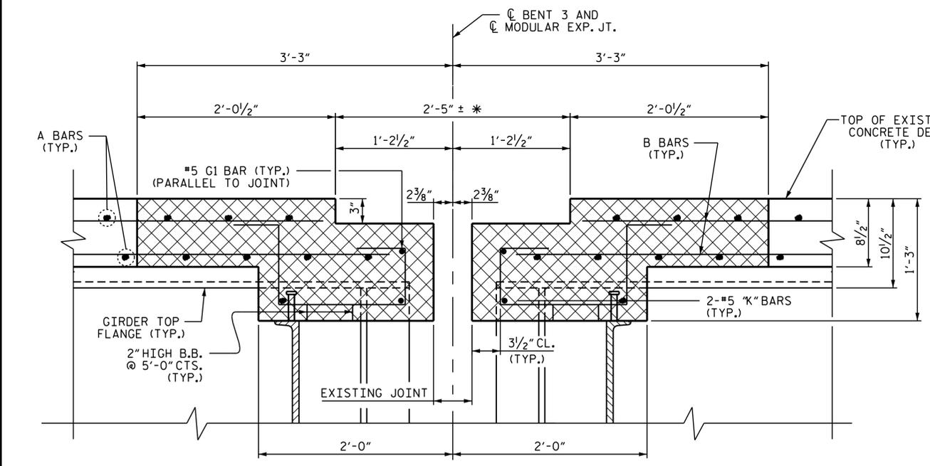
CONCRETE AND REINFORCING STEEL REPLACEMENT SECTION D-D
