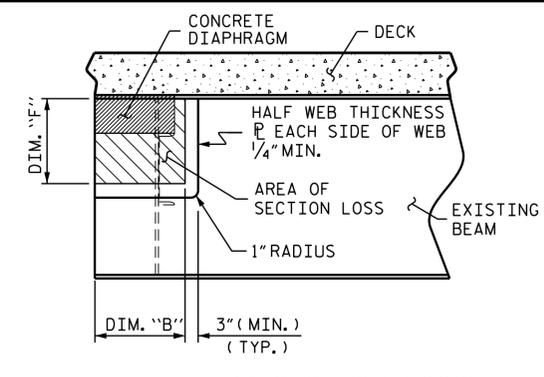
**BEAM END SECTION LOSS AND PLATING REPAIR**
