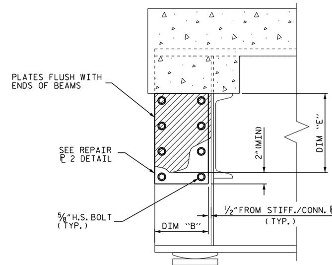
**BEAM END SECTION LOSS PLATING REPAIR**
