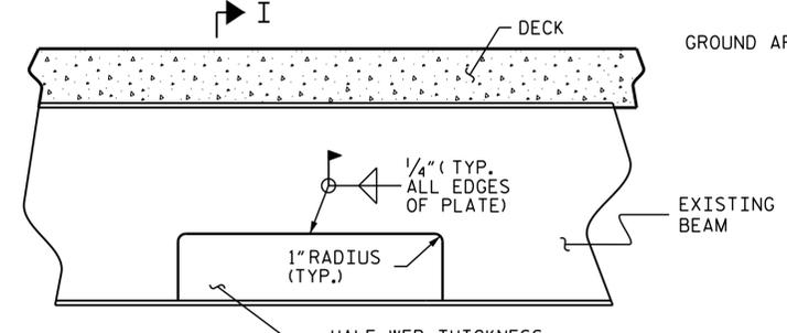
**INTERMEDIATE SECTION LOSS BEAM PLATING REPAIR**
