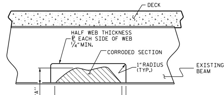
**INTERMEDIATE SECTION LOSS BEAM PLATING REPAIR**
