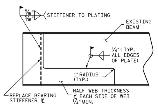
**BEAM END PLATING REPAIR**
