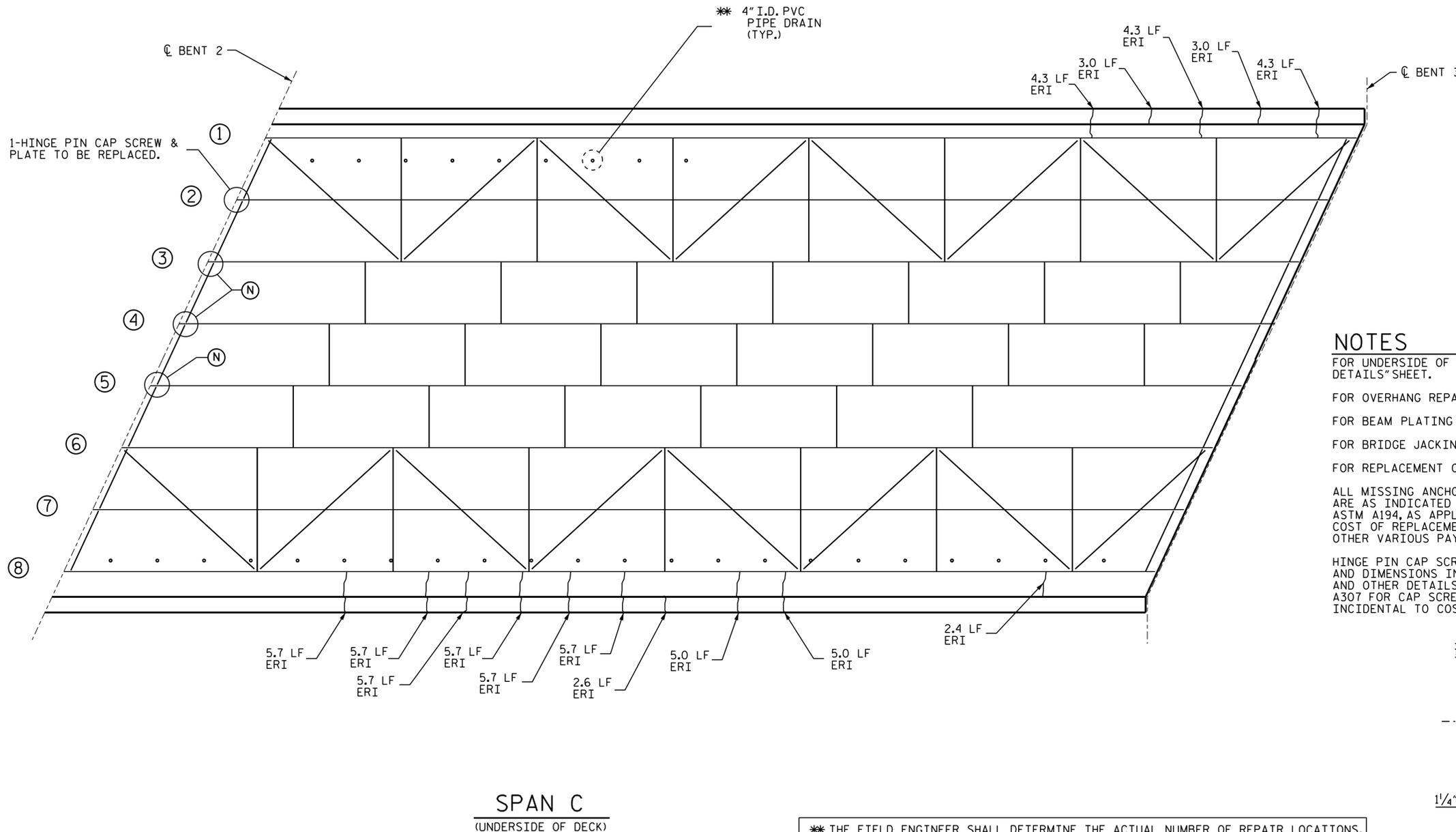
\* THE FIELD ENGINEER SHALL DETERMINE THE ACTUAL NUMBER OF REPAIR LOCATIONS. 11 LOCATIONS NOTED DURING FIELD EVALUATION. ESTIMATE QUANTITY, 1.1 CF OF SHOTCRETE EACH LOCATION ADDED TO "UNDERSIDE OF DECK" IN QUANTITY TABLE.
