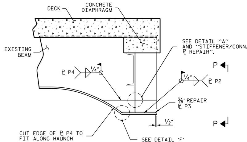
**BEAM END PLATING REPAIR**
