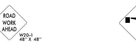
PLACED 500' IN ADVANCE OF FLAGGER. PLACED 250' IN ADVANCE OF FLAGGER.
