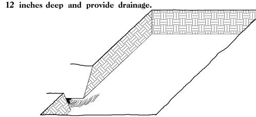
3. Backfill the trench with 2 inches well rotted sawdust. Place a 2 inch layer of well rotted sawdust at a sloping angle at one end of the trench.
