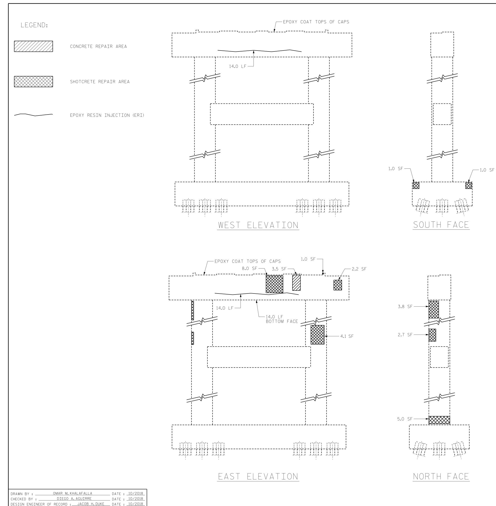
AS-BUILT REPAIR QUANTITY TABLE QUANTITIES ESTIMATE ACTUAL SHOTCRETE REPAIRS 13.2 CAP/FOOTING COLUMN/PILE 15.6 AREA SQ.FT VOLUME CU.FT. CONCRETE REPAIRS 3.5 ₩ CAP 1.8 EPOXY RESIN INJECTION LIN. FT. LIN. FT CAP 42.0 COLUMN/PILE PILE REPAIR JACKET LIN. FT. LIN. FT. INTEGRAL PILE JACKET AREA SQ. FT. EPOXY COATING CAP 120
