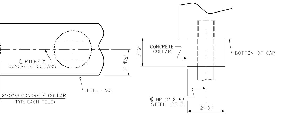
PLAN ELEVATION CORROSION PROTECTION FOR STEEL PILES DETAIL
