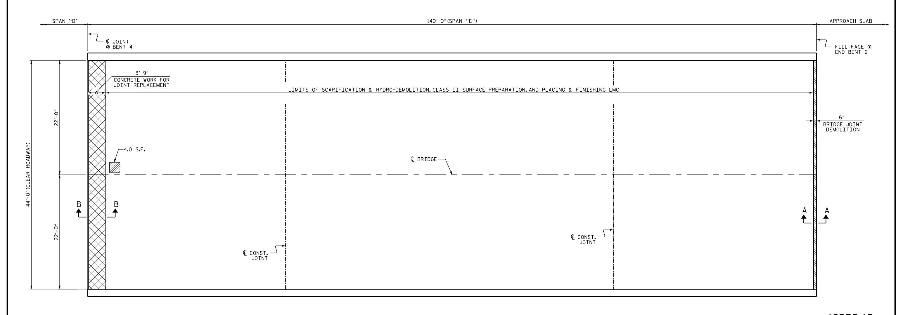
PLAN OF SPAN "E" - SCARIFYING BRIDGE DECK (SEE SHEET NO.S-10 FOR SECTION A-A AND SHEET S-11 FOR SECTION B-B) APPROX. AREA CLASS II SURFACE PREPARATION CONCRETE WORK FOR JOINT REPLACEMENT BRIDGE JOINT DEMOLITION
