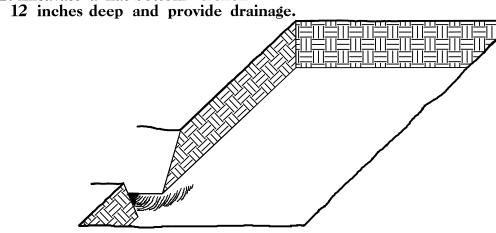
3. Jackfill the trench with 2 inches well rotted sawdust. Place a 2 inch layer of well rotted sawdust at a sloping angle
