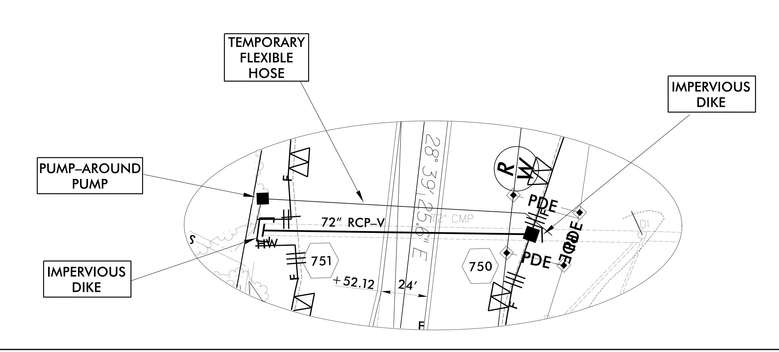
SEQUENCE OF CONSTRUCTION FOR TYPICAL WORK AREA: 1. UTILIZE STILLING BASIN(S) AS DIRECTED TO DEWATER THE WORK SITE.
