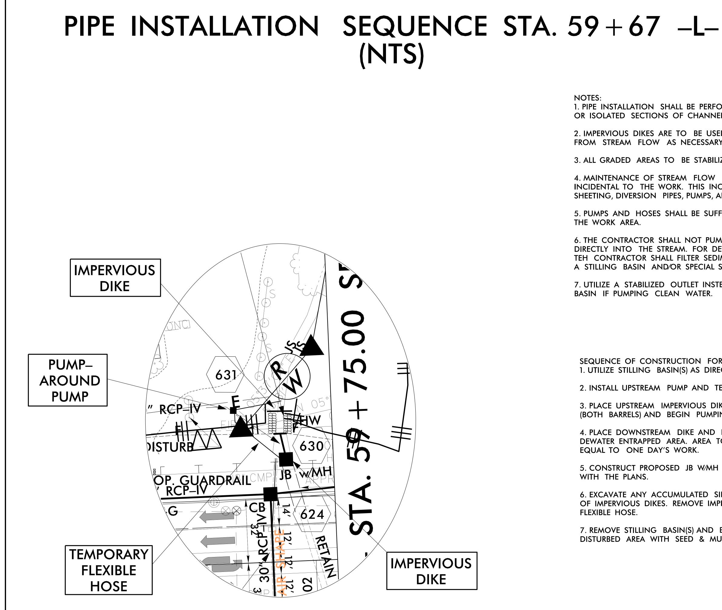
NOTES: 1. PIPE INSTALLATION SHALL BE PERFORMED IN ONLY DRY OR ISOLATED SECTIONS OF CHANNEL.
