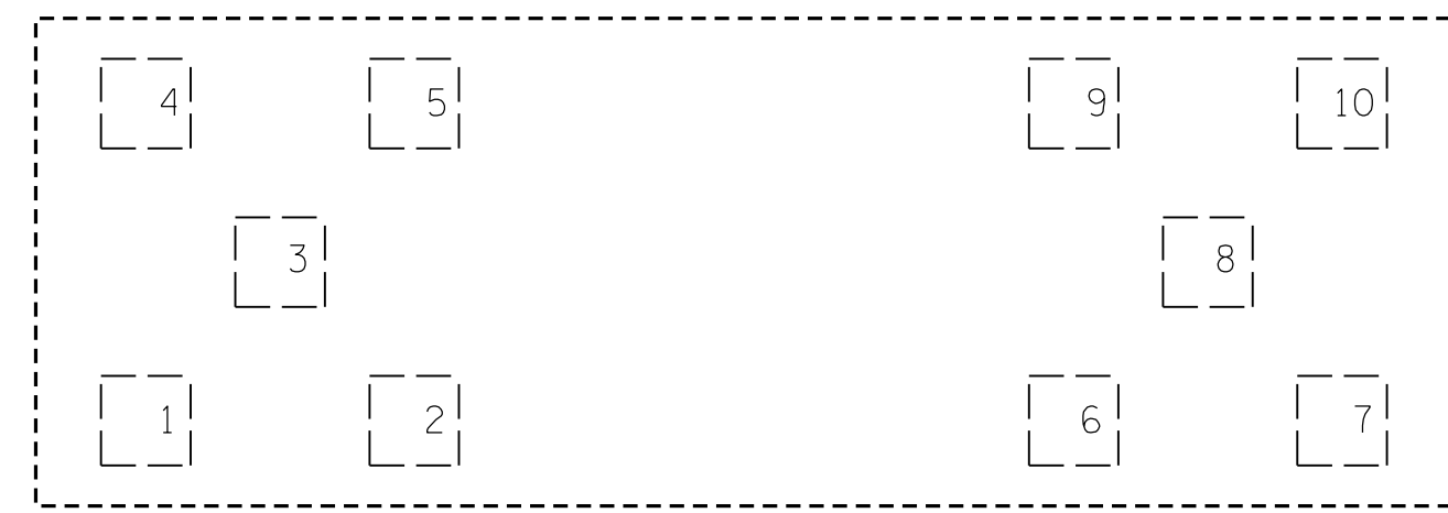
SEC A-A (NUMBERING OF PILES)
